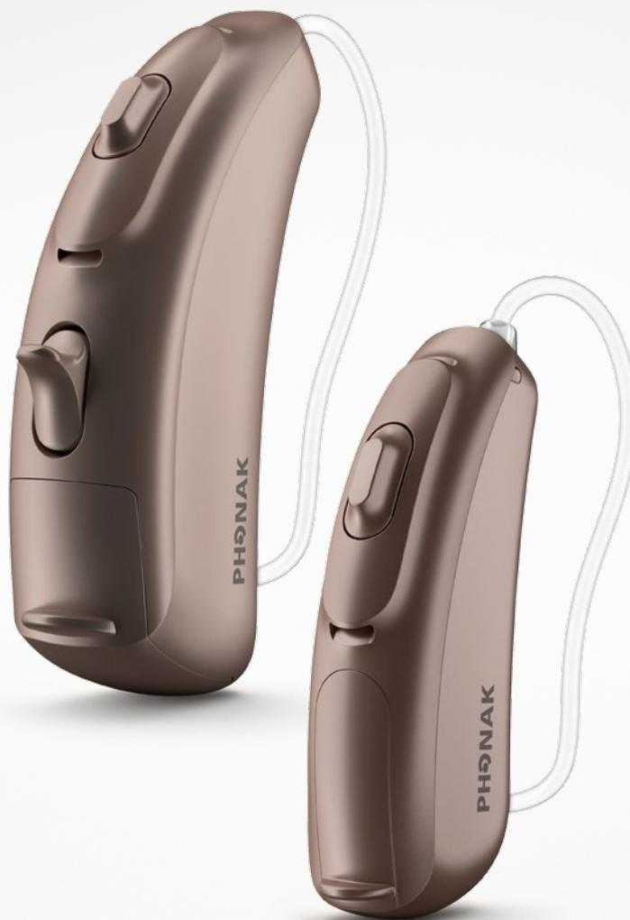
Phonak CROS B is a product for clients with an unaidable hearing loss in one ear. It is worn on the unaidable ear in combination with a Belong™ hearing aid on the better ear. CROS B transfers the microphone input signal to the hearing aid. The hearing aid receives the signal and plays it into the better ear to make sounds coming from the unaidable side audible. CROS B has no acoustical output.
